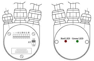
Three cables connect the rotary encoder. The power supply is achieved with a two-wire connection cable through one PG9. Each one of the twisted-pair and shielded bus lines are guided in and out through two PG9 on the right side (as seen on clamps). We strongly recommend to use the appropriate shielded and twisted cables.
