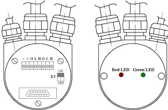
Three cables connect the rotary encoder. The power supply is achieved with a two-wire connection cable through one PG9. Each one of the twisted-pair and shielded bus lines are guided in and out through two PG9 on the right side (as seen on clamps). We strongly recommend to use the appropriate shielded and twisted cables.
